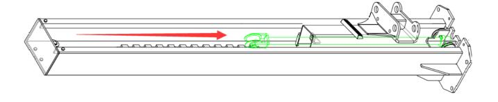
STEP 5 Install the hardware into top plate onto the top of the columns.
