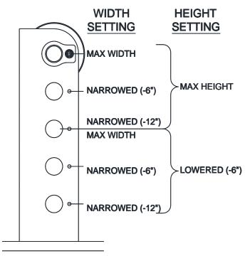
Fig. 3 - Sheave Position in Lower Bracket
