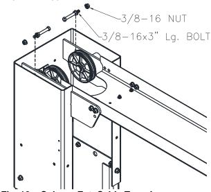
Fig. 10 – Column Ext. Cable Trapping
