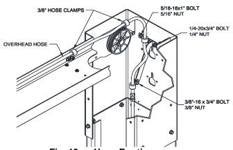
Fig. 13a – Hose Routing, Idler Side Column Ext.
