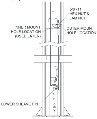
Fig. 2 – Cable Routing LAYOUT
