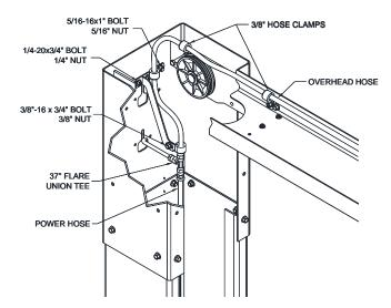
Fig. 13b – Hose Routing, Power Side Column Ext.
