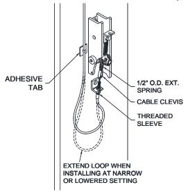
Fig. 16 - Idler Column Lock Assembly
