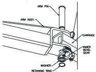
Fig. 17 -Arm Pin Keeper Install
