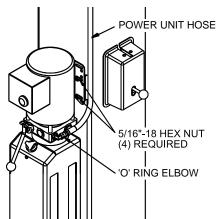
Fig. 12 - Power Unit Mounting
