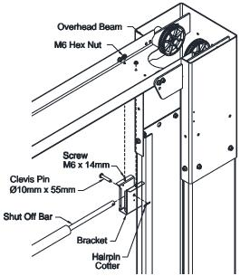
Fig. 9b – Overhead Bracket Idler Side
