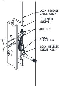
Fig. 15 - Power Column Lock Assembly
