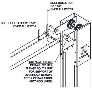
Fig. 8 – Overhead Assembly
