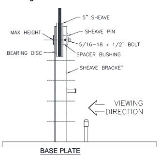
Fig. 4 – Sheave Assembly and Cable Routing
