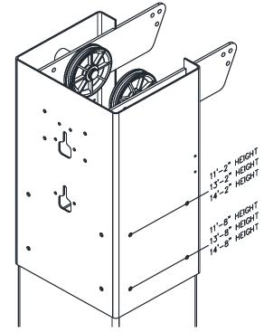
Fig. 5 – Column Extension Assembly
