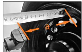
Measure the distance between wheel and gauge index
