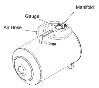
Figure 2 - Air Tank Replacement Parts
