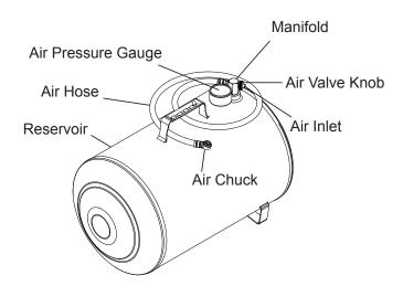
Figure 1 - Typical Air Tank Nomenclature
